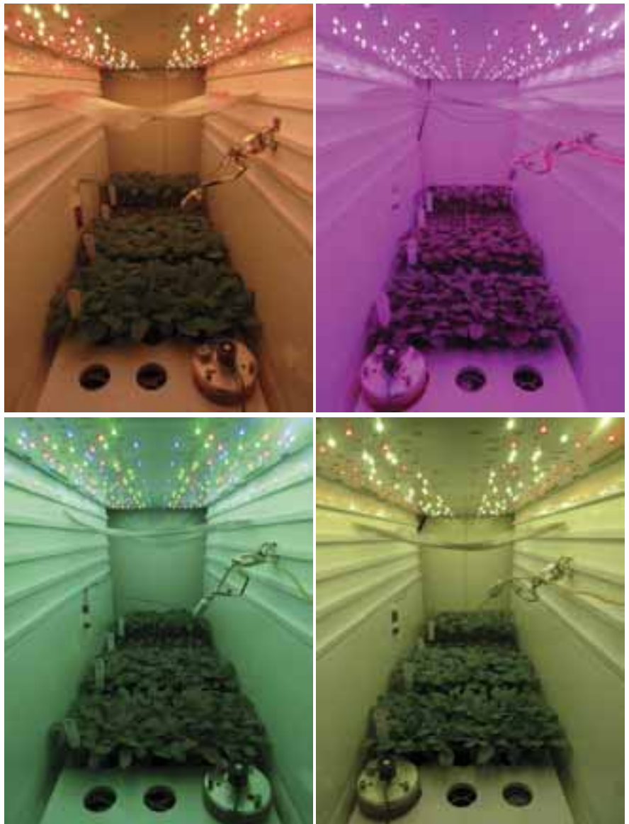
Figure 2. Research being performed with ornamental transplants inside custom-designed LED growing modules at Michigan State University.
